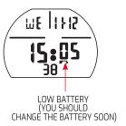
If the flashing battery (icon) appears on the display, the dive functions are disabled for safety
