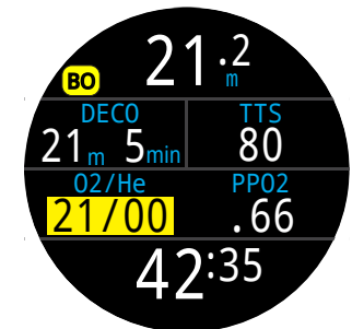
14. Gas Switch Required
